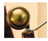
Step 2 Insert claw/screwdriver between metal caster collar and plastic socket.
